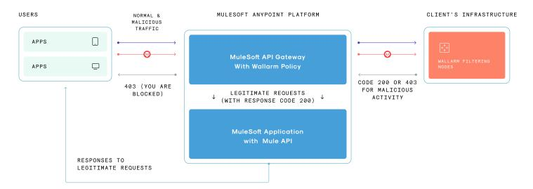
This configuration allows anonymized traffic to be routed to the external Wallarm node for analysis and protection against potential threats. Through this approach, Enterprises can ensure effortless integration, secure traffic analysis, risk mitigation, and the overall enhancement of their App and API security.
